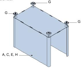
Carefully, lift the battery and slide it inside the enclosure from the top.
